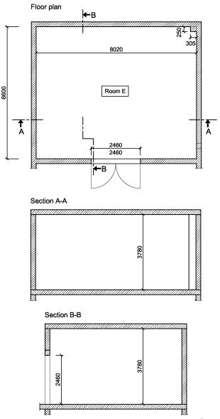
Figure C.1 shows the drawings of the reverberation room.
